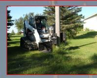
Remove poles safely and comfortably from inside the machine.
