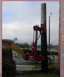
Capable of removing poles up to 90 feet in length.
