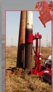
Two large 3x6 inch clamp cylinders and metal teeth on the jaws securely hold pole in place during extraction. Call us Toll-Free at 1-877-433-5733 www.ezspotur.com
